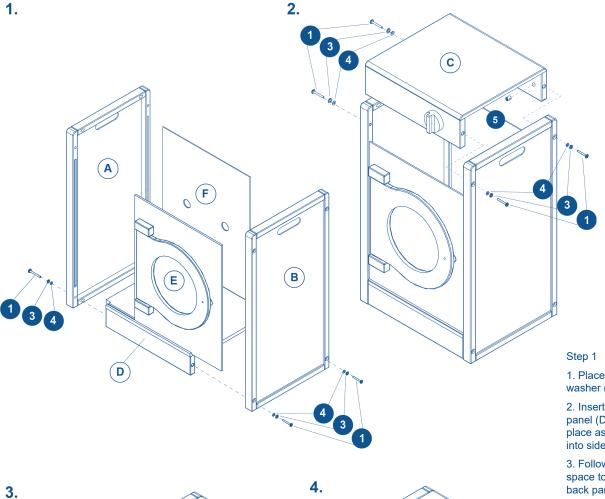
1. Place flat washer (4) and lock washer (3) on large screw.
