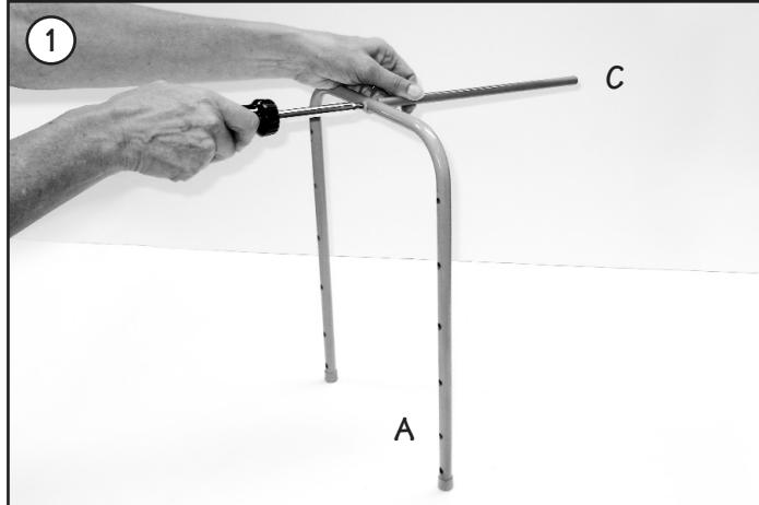
2. Attach other 2 connecting rods **C** to bottom of the same side frame **A** by using a large bolt through the bottommost holes on both legs of the side frame.
